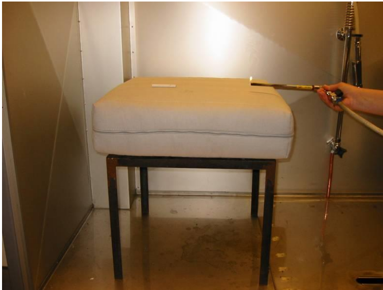
Figure 5 Test set-up according to BS6807
